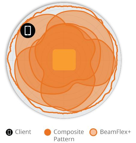
Figure 2. R500 2.4GHz Azimuth Antenna Patterns
