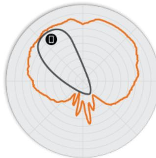
Figure 5. R500 5GHz Elevation Antenna Patterns
