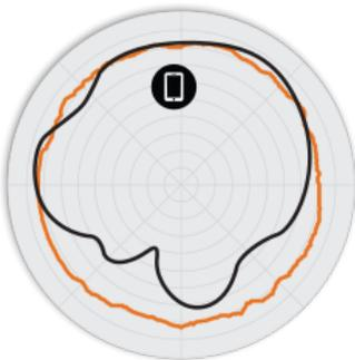
Figure 3. R500 5GHz Azimuth Antenna Patterns
