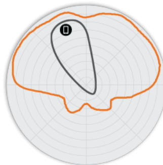
Figure 4. R720 2.4GHz Elevation Antenna Patterns
